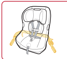
Finished Lower Anchor Belt Routing
